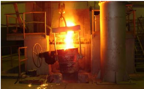
**Fig. 6** Teaming of liquid melt into the one-ton ladle.
