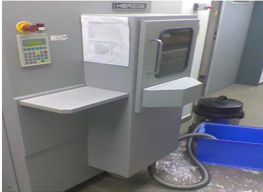
**Fig. 3** Spectro analytical instrument used to polish cast or rolled material prior to the determination of the chemical compositions.
