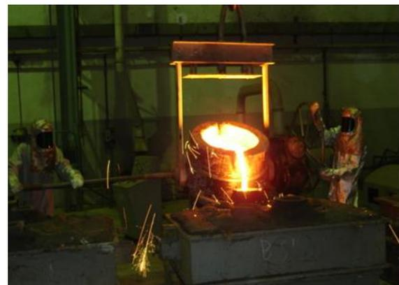
**Fig. 7** Casting of roof hangers.
