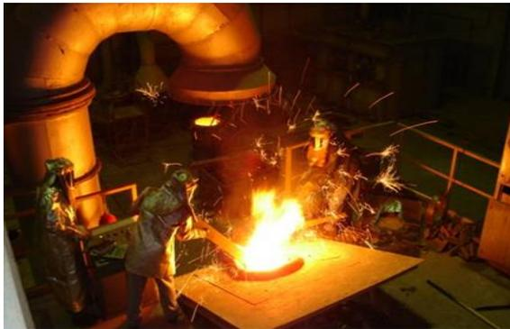
**Fig. 5** De-slugging process at the one-ton induction furnace.
