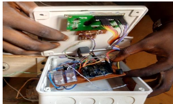
Fig. 7 Components mounted in casing.
