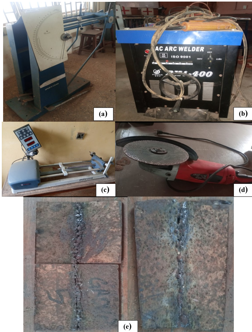
Fig. 1 Setup for (a) Chappy test machine, (b) electric arc welding machine, (c) tensile test machine, (d) grinding machine, and (e) workpiece.
